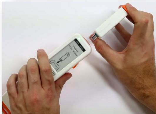
7. Insert the strip into the port on the top of the mx3 lab with the blue label facing upwards, then release the button
